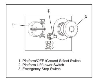
Figure 3-1. Ground Control Station
