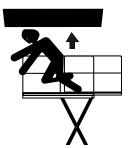
• During operation, keep all body parts inside platform railing.
