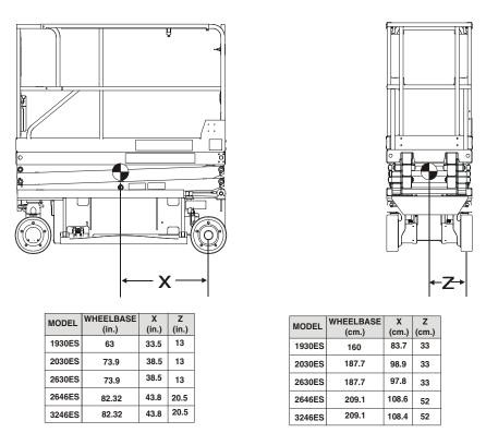
Figure 4-7. Lifting and Tie Down Chart
