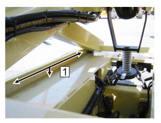
Figure 6-2. Lower Slide Pad Channel
