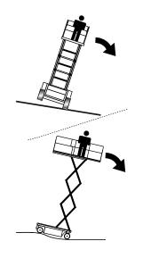
• Do not elevate platform or drive with platform elevated while on or near a sloping, uneven, or soft surface. Ensure machine is positioned on a firm, level and smooth surface before elevating platform or driving with the platform in the elevated position.
