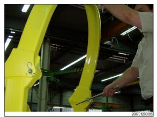
Both sides must be secured with bolts and split pins during operation.
