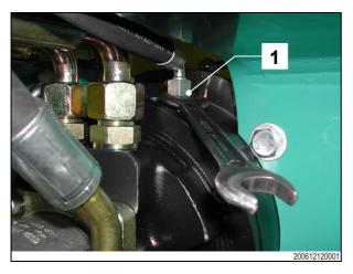
Remove the brake hose (1) from the front roller drum drive motor.
