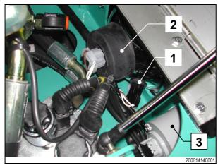
Open the front hood; this will allow you access to the parking light from the inside (1), as well as to the dipped headlights (2) and the indicators (3).
