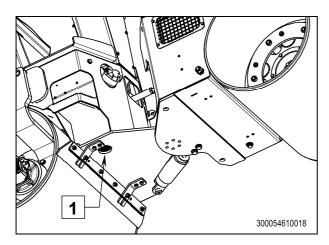
Unscrew the screw (1) under the roller using a square socket wrench (13 mm). You can find this wrench on the ratchet of the socket wrench set.
