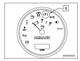
Start the machine. The brake light (P) (1) must extinguish quickly. Test the forwards and the backwards drive.
