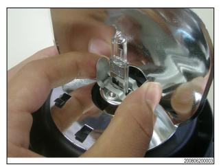
Press the two lugs of the bulb holder together.
