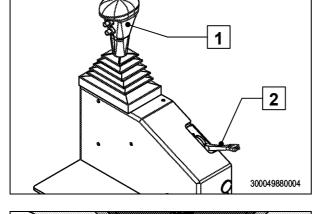
Now turn the emergency stop button (1) slightly in the direction of the arrowuntil it disengages.
