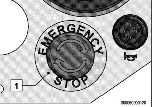
Release the emergency stop button by pulling upwards in the "pullpush" version. The direction arrows are missing from this button.
