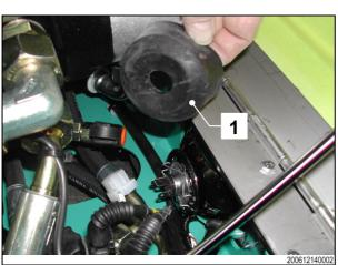
Press the end of the bracket (1) to remove it.
