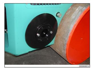
If one of the two disks is not being used fix it to the mounting provided on the right of the roller.
