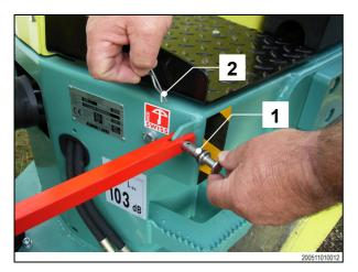
Now snap in the joint protection and secure it with the lock bolt **(1)**.
