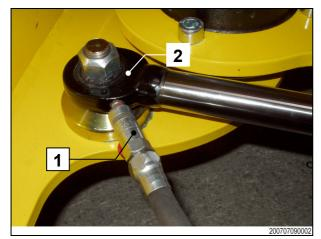
Clean the grease nipple before greasing.
