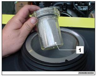
The plastic water filter container (1) can be stored on the machine, in the water tank water filter.
