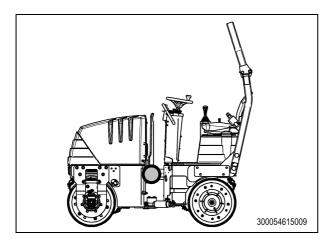
The center of gravity relevant to transport is located 670 mm from the floor and approx. in the center of the machine, depending on the fill level of the diesel or water tanks.
