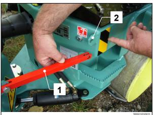
Carefully turn the roller steering wheel until the joint protection **(1)** comes in line with the opposite loop **(2)**.
