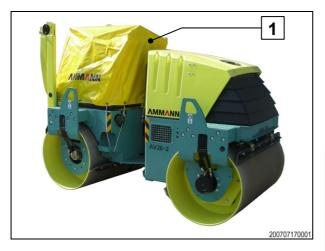
The driver's platform and the instrument panel can be protected from dirt and water using the driver's platform cover **(1)**.
