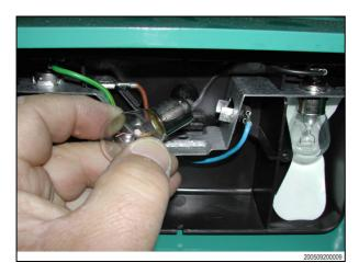
Replace the defective bulb with a new one of the same type and power.
