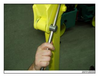
Fit the two bolts and split pins. You may need to use a bar to tighten the bolts.
