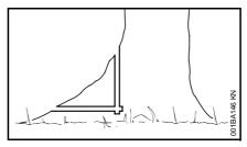
Remove large buttress roots: Make vertical cut first, then horizontal – but only if wood is sound.
