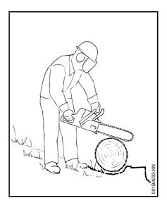
If on a slope, stand on the uphill side of the log. Watch out for rolling logs.
