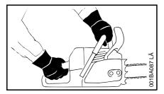
Always hold your saw firmly with both hands – right hand on the rear handle, even if you are left-handed. To ensure safe control, wrap your fingers tightly around the front handle and control handle.
