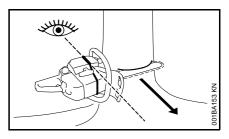
When making the felling notch, make use of the gunning sight on the shroud and housing to check the planned direction of fall.
