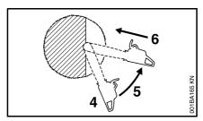
Begin cut (4) by applying lower portion of the guide bar nose – do not use upper portion because of risk of kickback. Cut until depth of kerf is twice the width of the guide bar.
