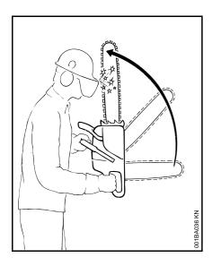
Kickback occurs when the saw is suddenly thrown up and back in an uncontrolled arc towards the operator.
